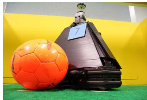
Fig. 1 Soccer robot of Hibikino-Musashi Team for the Robocup Middle size league
